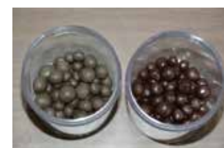
Fig.7 Melted spherical aggregate using dehydrated cake from crushed stone quarry
