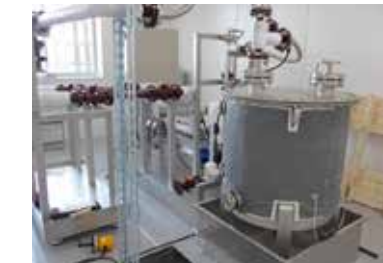
温泉模擬実験装置 Laboratory test facility simulating hot-spring
