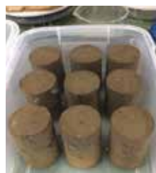
Fig.2 Drying and wetting test using Fiber-cement stabilized soil
