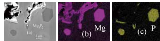
Fig.2 Mg phosphide in Al : SEM view (a)and mapping (b,c)
