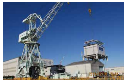
Fig.3 The marine transportation of device from Sakai factory of Hitach Zosen Corporation (Task1 / Wave power generation)
