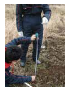
Fig.5 In situ test to measure ground strength property using developed test device
