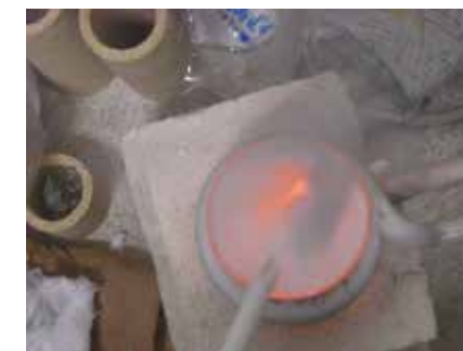
Fig.4 Photograph of inductively heated NaCl-KCl molten salt by application of RF (400kHz) EM field energy.
