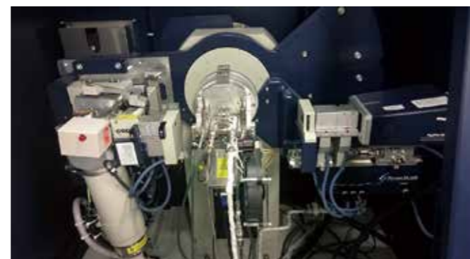
Fig.2 High temperature X-ray diffractometer with 2-dimensional detector.
