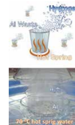
Fig.4 New hydrogen production method using hot spring water.
