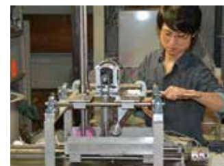
Fig.1 Developed apparatus to continuously recycle high-water content mud generated from disaster sites
