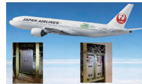
Fig.4. Boeing 777-200ER aircraft and two equipments for atmospheric observation installed in her cargo room.
