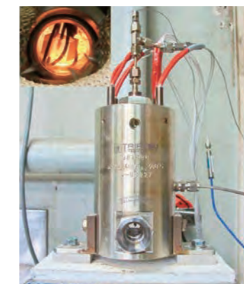
Fig.2 Visible-type autoclave for observation of hydrothermally derived fracturing by decompression at high temperature.
