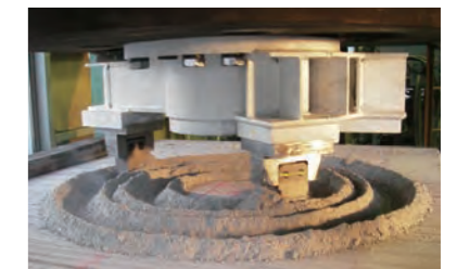
Fig.7 Experiment of cutting reinforced concrete using specially developed bits
