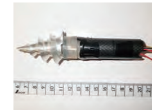
Fig.8 Curvable small diameter drilling machine for ground survey
