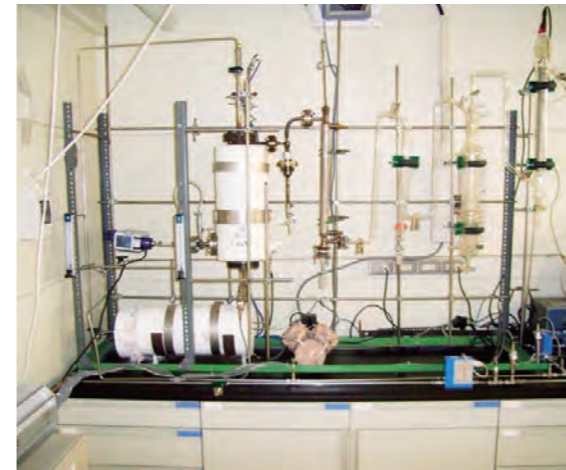
Fig.2. Fluidized bed plant.
