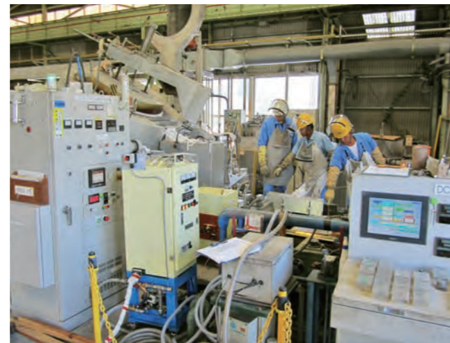
Fig.1 Electromagnetic hydro-cyclone separator system for removal of inclusion particles from molten aluminum.
