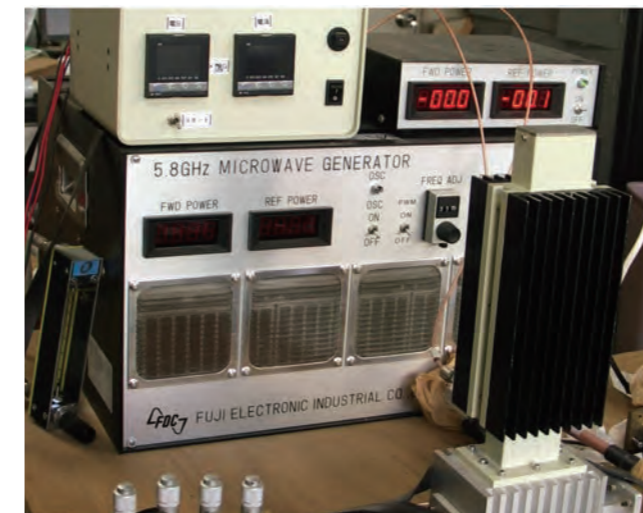
Fig.2 5.8GHz Semi Conductor Microwave Generator.
