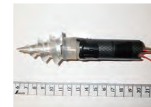
Fig.8 Curvable small diameter drilling machine for ground survey
