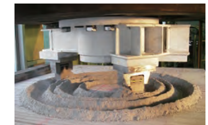
Fig.7 Experiment of cutting reinforced concrete using specially developed bits
