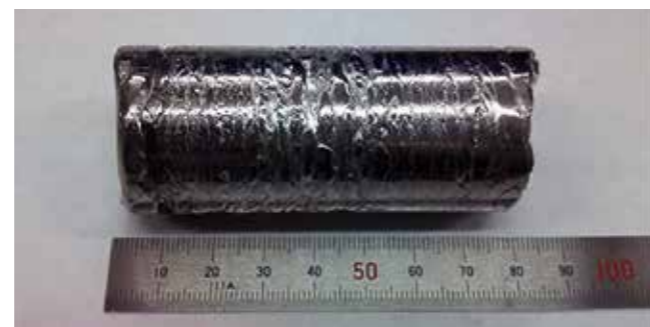
Fig. 2 Appearance of a Mosibitic alloy produced by a plasma-melting technique.
