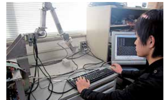
Fig.7 Experimental apparatus to judge the existence of obstacle by resistive forces acting on the bucket
