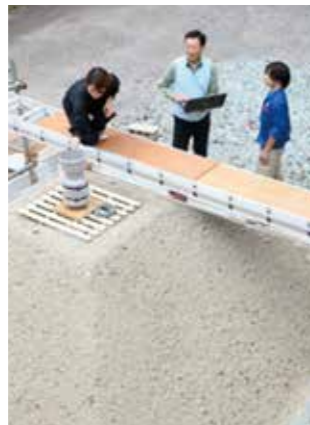
Fig.1 Embankment to examine the durability for erosion by rainfall
