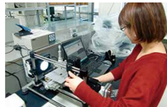
Fig.5 Measurement wetting property of insect cuticle
