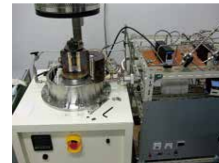
Figure 2. Equipment for measuring elastic modulus of ceramic materials by a resonance method at elevated temperatures under controlled atmospheres.
