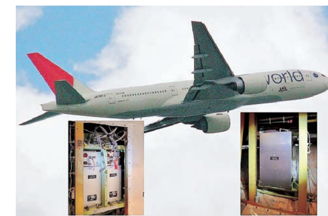
Boeing 777-200 and two equipments for atmospheric observation installed in her cargo room.
