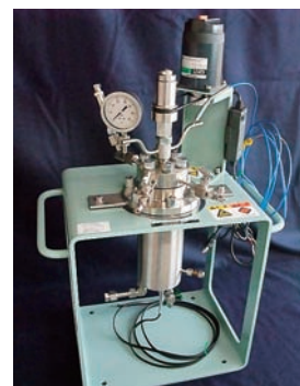
Fig.2: New reactor enabling rapid heating and cooling in the hydrogen production experiments.
