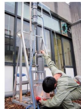
Fig.4 Jet test to investigate durability for the erosion of fiber-cement-stabilized soils.
