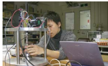
The developed experimental device to evaluate adhesion between soil and metallic material.
