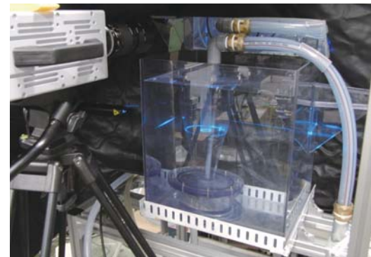
Fig.1 Flow measurement by particle image velocimetry in cyclone system.
