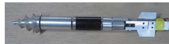
A prototype of mole robot for ground survey.
