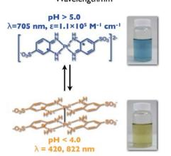
Figure 2 pH-Responsive Switching of the Near-Infrared Absorption of the Water-Soluble Bis(o-diiminobenzosemiquinonato)platinum(II)
