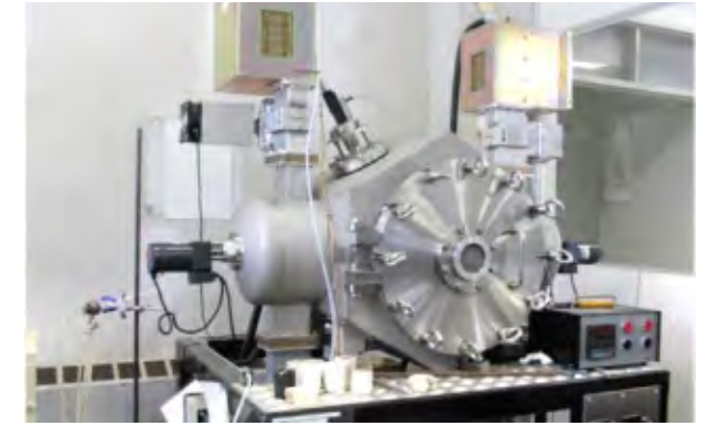
Fig.3 7-kW multi-mode microwave furnace used for metal recycling from wastes.
