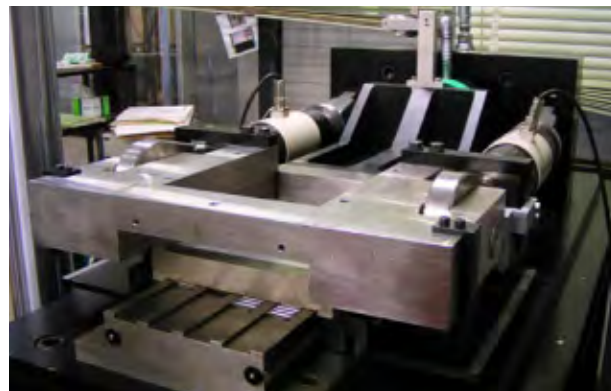
Fig.1 Photo of direct shear test apparatus
