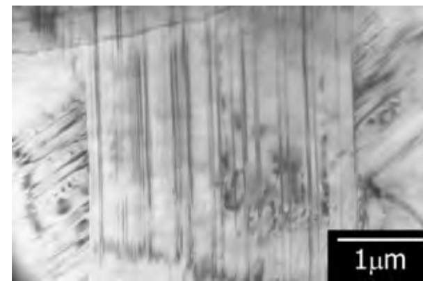
Fig.3 TEM microstructure of the LPSO (Long Period Stacking Ordered) type \text{Mg}_{85}\text{Y}_9\text{Cu}_6 alloy.
