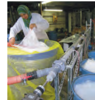
The improved experimental apparatus for cuttings transport by foam. The inner pipe rotates.
