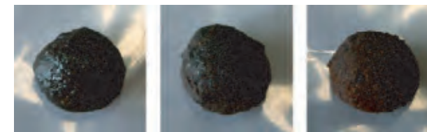
Some heated samples obtained by melting mixture of dehydration cake and other wastes.
