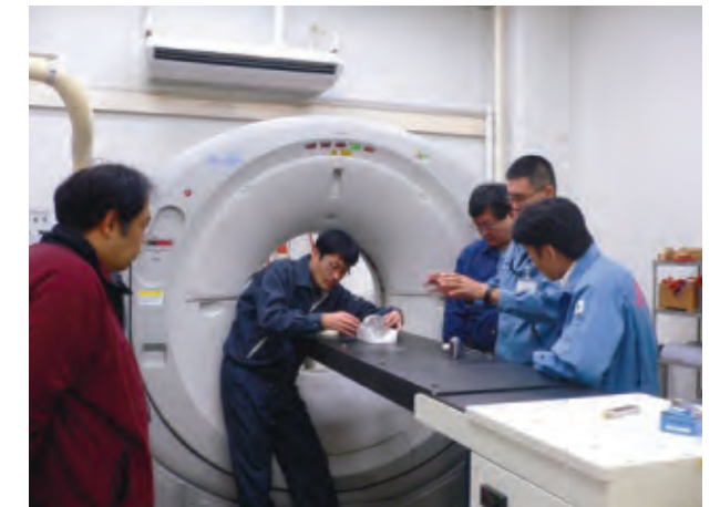
Fig.2 X-ray CT Measurements for Fractured Rock Core at JOGMEC
