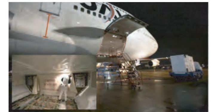
Boeing 747-400 and two equipments for atmospheric observation installed in her cargo room.
