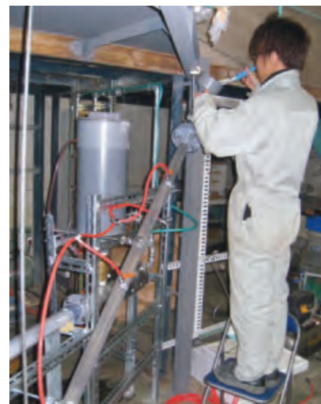
The experimental device to separate soil from crushed asphalt under grizzly, using free fall and spiral flow.
