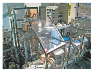
Figure 1 Continuous flow reactor for partial upgrading of bitumen by
