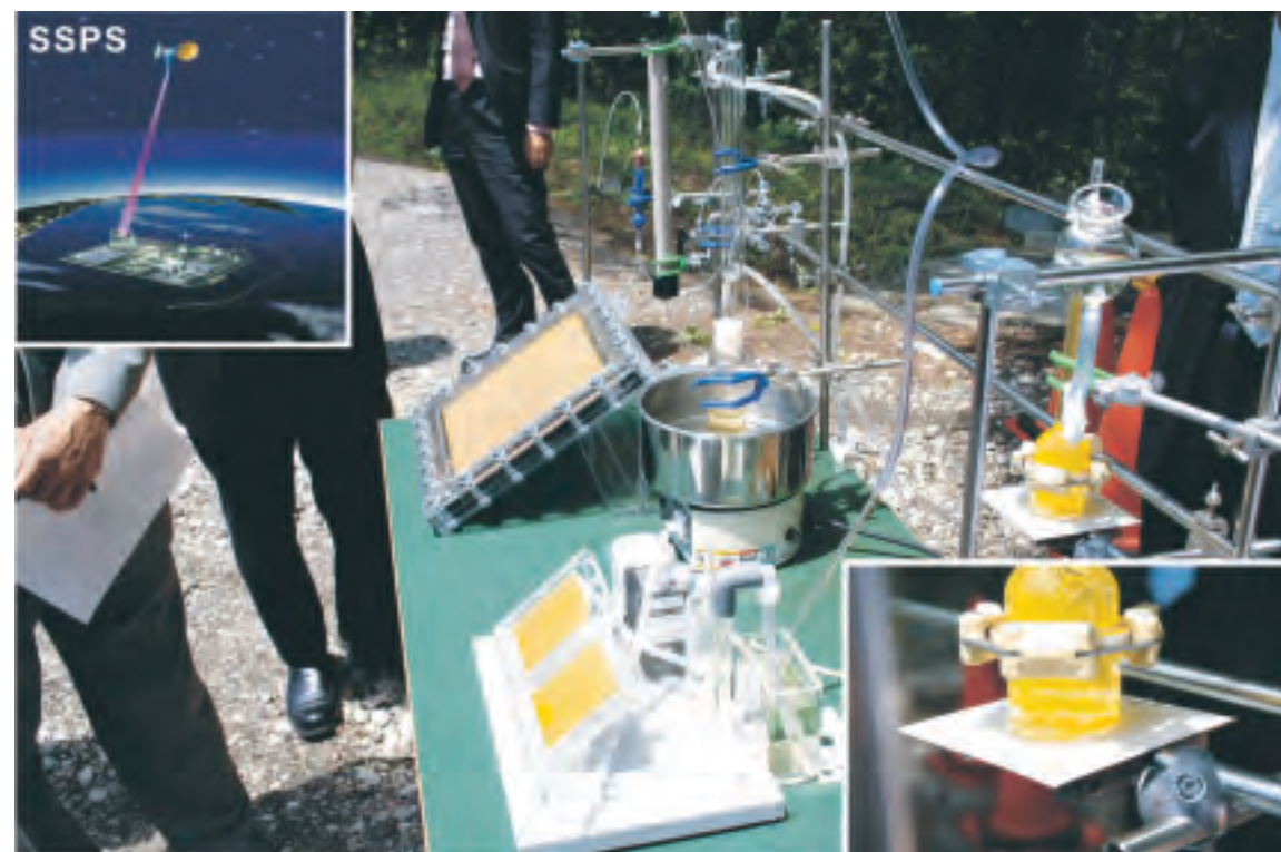
Demonstration of hydrogen generation experiment using solar light. Left upper inset is illustration of Laser Space Solar Power Systems (L-SSPS). Right lower inset is picture of hydrogen generation reactor.
