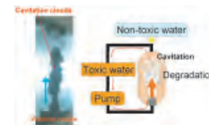
Schematic diagram of degradation of toxic compounds with cavitation induced by submerged waterjets.
