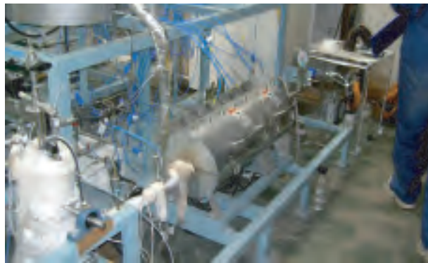
Fig.1 Tube type continuous reactor for partial upgrading of bitumen by supercritical water.
