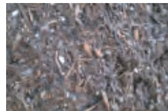
Fiber-stabilized soil mixed with wood-chips after the test
