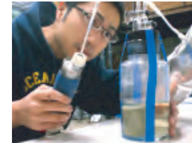
Measurement of a concentration of hydrogen sulfide generated from the modified soil
