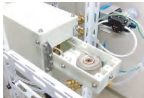
Fig.1 : Metal droplet generator with intermittent electromagnetic force imposition.
