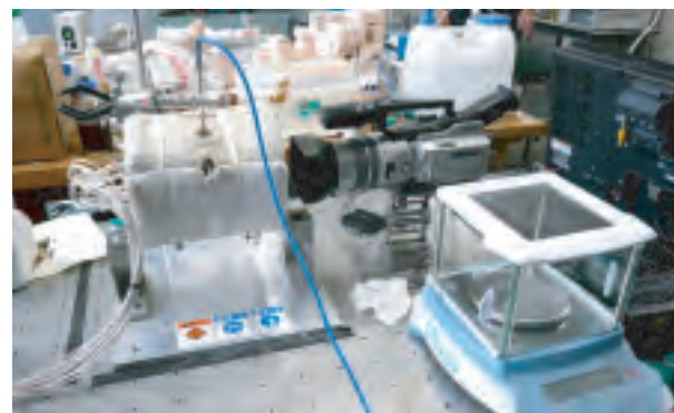
Fig.3 Experimental equipment I: pressure vessel with optical windows.
