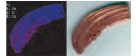
炭酸カルシウム堆積物の断面 Cross section image of calcium carbonate sedimentation. Ca/Fe alternative layer is observed by XGT image.
