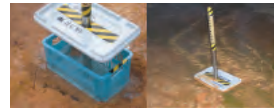
温泉での炭酸カルシウム堆積の様子（右は左の写真の約4ヶ月後） Appearance of calcium carbonate sedimentation in hot spring (Right photograph is about four months after the left photograph). Okuokuhashikuro hot spring, Akita).
